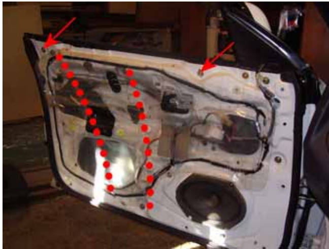
Fig 5. Window guide rails and stopper locations
