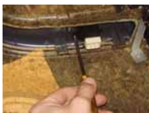
Fig 4. Removing window control
